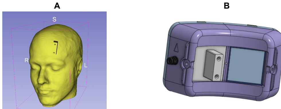
Figure 1: (a) Rendering of the mannequin with a slot for positioning the transducer and (b) transducer housing with extrude that fits into the slot.
